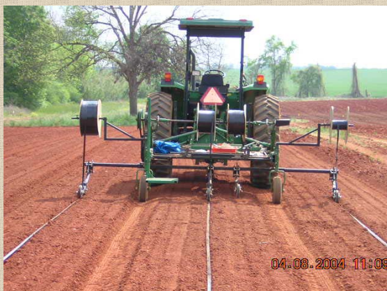
Figure 3: Drip tubing installation for 0.91 m and 1.83 m.
