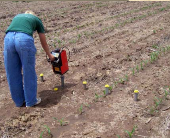
Soil water readings by neutron probe in Plant 2 Skip 2 corn
