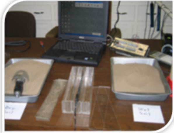
Fig. 2: Plastic box, sensor, datalogger & computer setup
