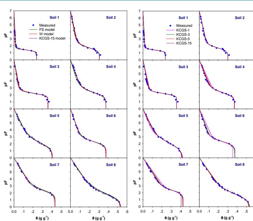
**Fig. 1 Comparison of the measured soil water retention curves versus the estimations from the FS model, W model and KCGS-15 model. The KCGS-15 model are established from water retention data of 0-1500 kPa.**
