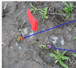
Figure 1. Plant Root Simulator TM -probes used to measure the effects of broadcasted liquid swine manure on soil nutrient availability (Photo courtesy of Dr. Ken Van Rees).
