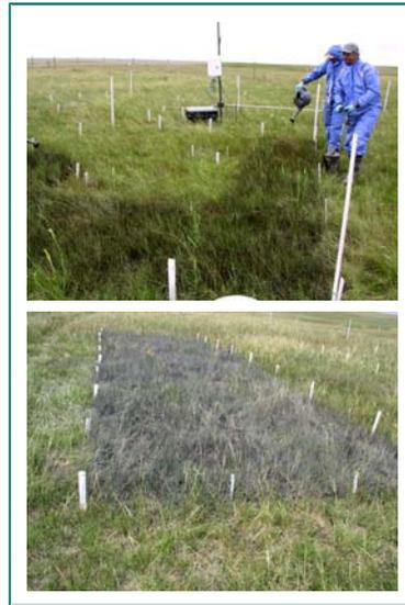
Figure 1. Top: drilling mud application using watering cans; below: plot after mud application.
