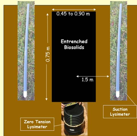
Figure 2: Instrumentation of trenches. Each trench was 15 m long.
