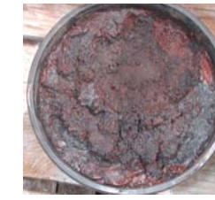
Figure 18. Uneven water infiltration in soil amended with high VM charcoal (22.5%)
