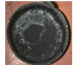
Figure 17. Water absorption in low VM charcoal (6.3%)
