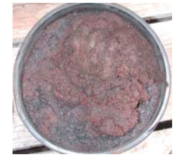
Figure 19. Uniform infiltration in soil amended with low VM charcoal (6.3%)
