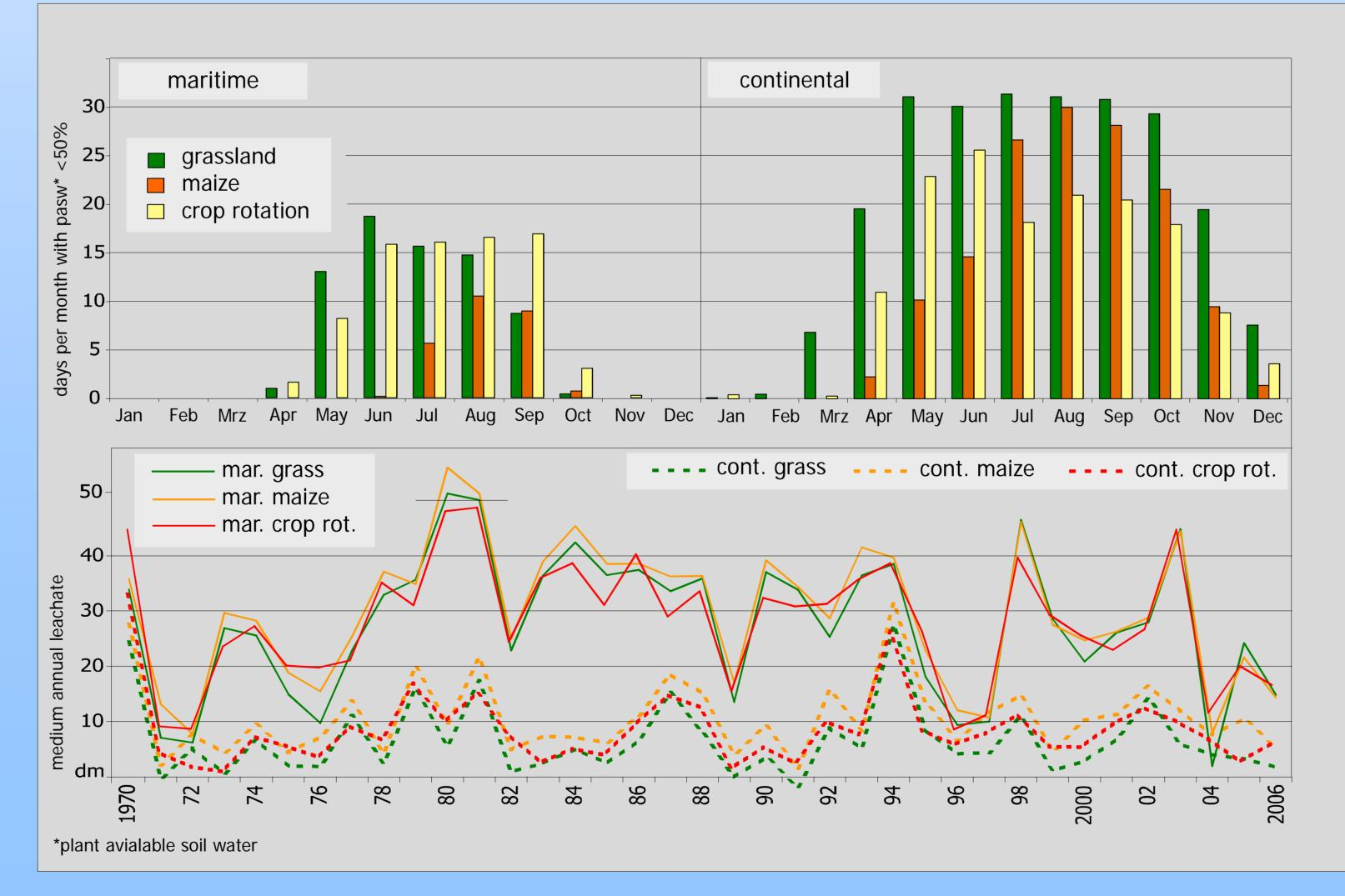
Fig. 4: Simulated soil water content and amount of leachate for the different energy production systems, averaged over 36 years.
