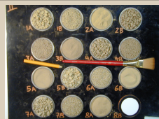
Figure 2. Size fractions, in 50mm diameter Petri dishes, that were scanned for several experiments related to aggregate stability and other soil properties including the 2 mm fraction for soil survey purposes.
