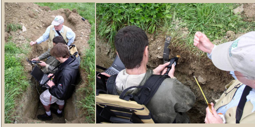
Figure 3. Pedon in situ measurement of hyperspectral reflectance by horizon.
