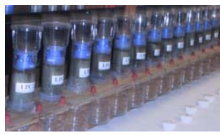
Fig. 2. Soil columns instrumented with leachate collection system
