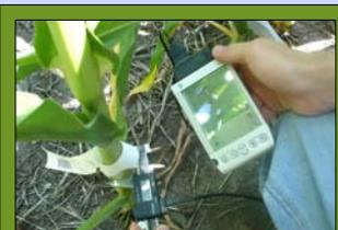
Measurement of R3 stalk diameter at the 6<sup>th</sup> internode on individual plants with use of a digital caliper and a Visor<sup>®</sup> personal data assistant.
