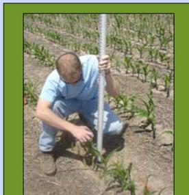
Measurement of V5 plant height on individual plants with use of a bar-coded height stick and a Symbol<sup>®</sup> personal data assistant.
