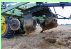
Paratill™ implement with typical shank arrangement (points facing inward).
