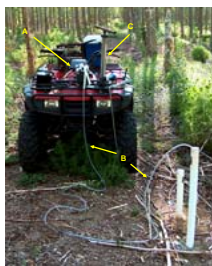
Figure 3: ATV used to collect pore water samples from porous cup lysimeters. A peristaltic pump (A) and length of clear vinyl tubing (B) was used to collect the samples. A bicycle type pump (C) was used to apply the vacuum.
