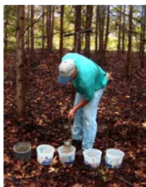
Figure 4: Soil Sampling sweetgum plots at depths of 0-5, 5-15, 15-30, 30-60, and 60-90 cm. Composite samples from 4-6 borings per plot were taken, half within row and half between row.
