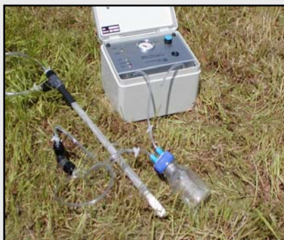
Figure 4: Suction lysimeter and pump to extract soil solution at a depth of 60 cm.
