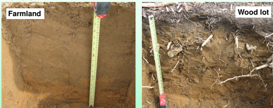
Fig. 1 Distinct soil profiles from the farmland and woodlot. Compared to the farm soil, the wood lot soil shows more clearly defined, darker, and thicker A horizon. Morphologically, the farm soil is more vertically homogenous than the woodlot soil.
