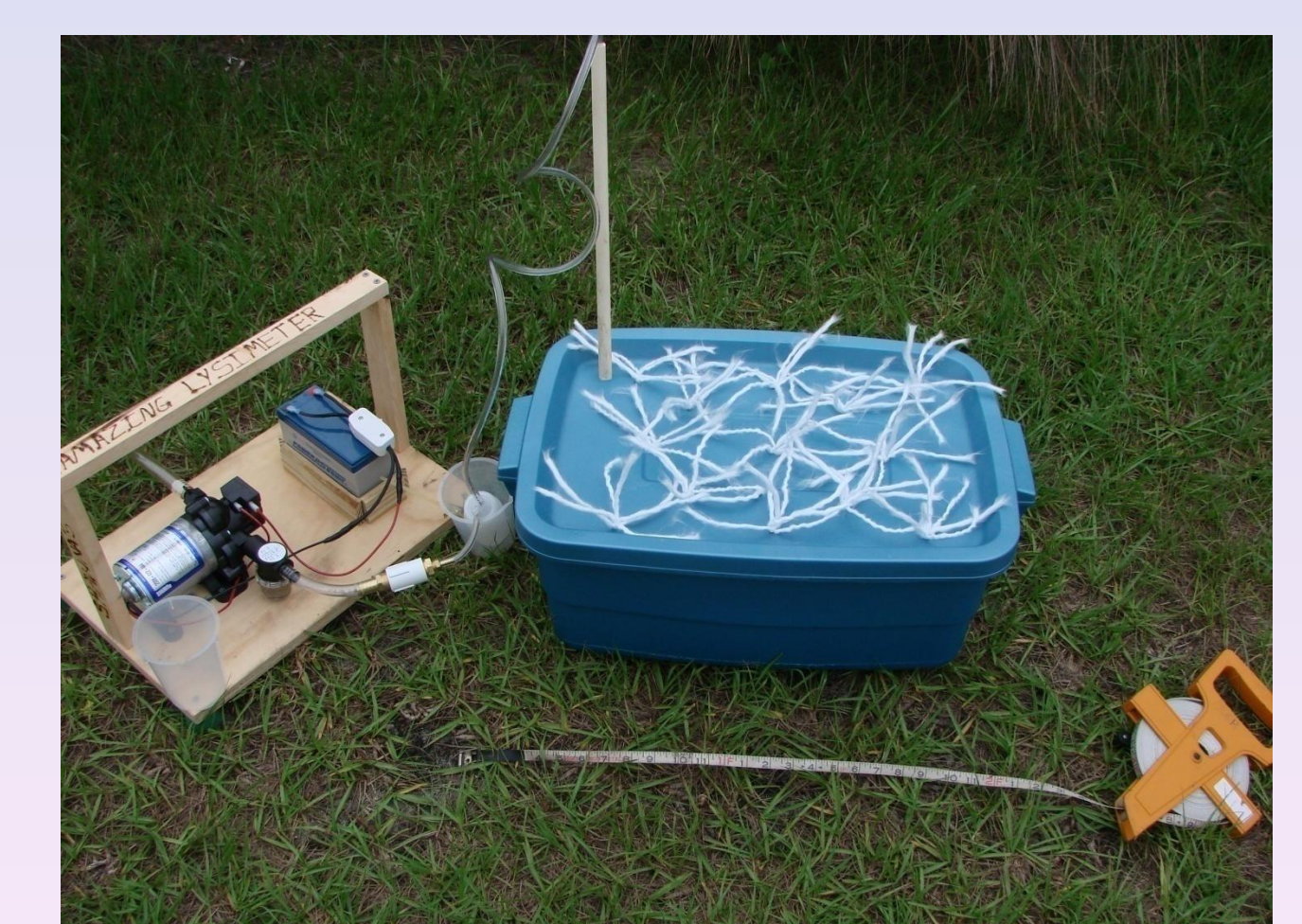
Fig. 7. A passive wick leachate collector that will be installed under simulated mixed landscape plots.
