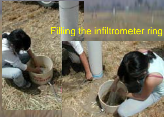
Marriott/reservoir supplies water and controls the head
