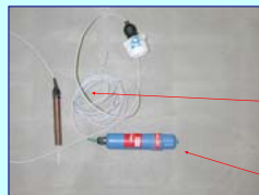
Marriott/reservoir supplies water and controls the head
