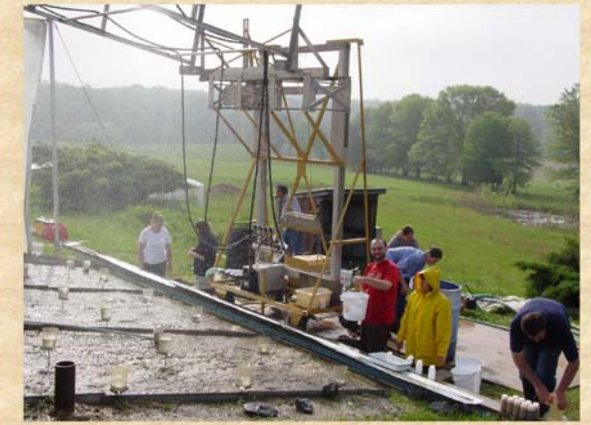
Rainfall simulation at the clay loam bare plot.
