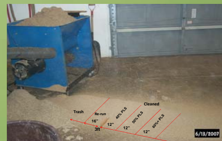
Cleaned seed is collected at a distance from 3 – 6 feet from the cleaner and ranged from 40 – 60% pure live seed with material harvested in 2007.
