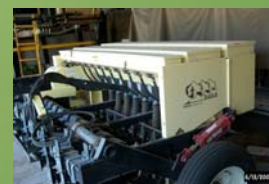
Cleaned seed is collected at a distance from 3 – 6 feet from the cleaner and ranged from 40 – 60% pure live seed with material harvested in 2007.
