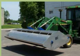
Airflow around the upward rotating brush pulls seed heads into the brush where seed are removed by flailing action and are propelled in the seed bin.
