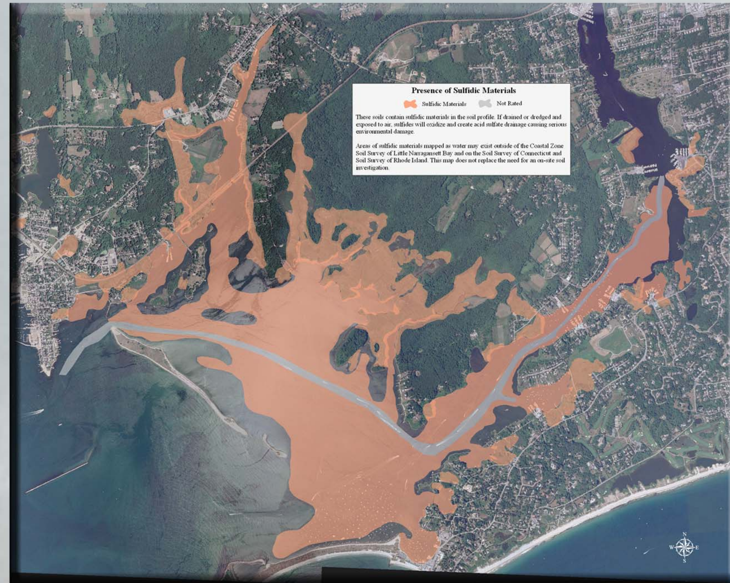
Figure 1 - A map identifying sulfidic materials, which when exposed to air produce sulfuric acid resulting in acid sulfate drainage. Habitat degradation and loss of biodiversity is caused by the release of acid and high concentrations of Fe, Al, Mn into the environment. If buildups of acid or dissolved ions occur, this can be extremely toxic to plants and animals. Development activities in sulfidic materials have resulted in marsh dieback, concrete corrosion and structural subsidence. This information would be beneficial in a coastal hazards atlas and important to SAV habitat restoration.
