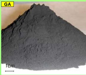
Fig. 4 Ash from thermal gasification of pig manure (a) and its particles seen under the microscope (b) (GA).
