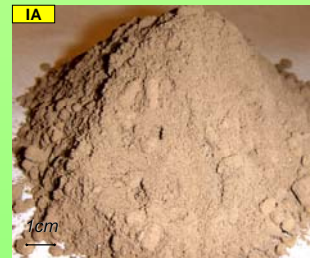
Fig. 5 Ash from incineration of pig manure at 1000°C after 24h (IA).
