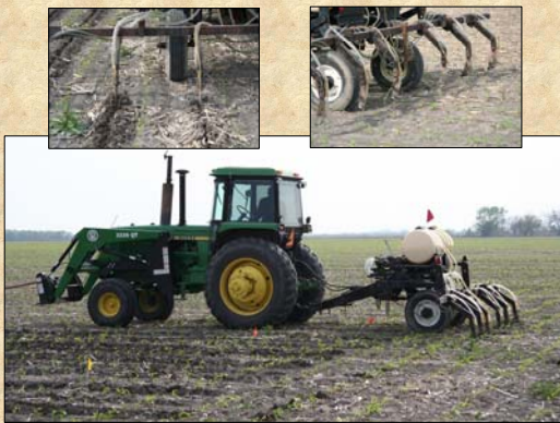
Plate 1. Liquid applicator used to apply N and P fertilizers at varying depths into Blackland soil. Thrall, TX.
