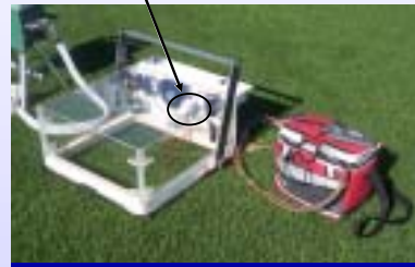
Figure 3. Large chamber fabricated to measure CO 2 fluxes in turfgrass. The system was connected to and controlled by a datalogger in the red cooler.
