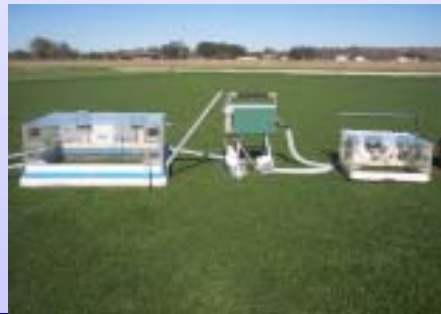
Figure 2. Large chambers cover surface areas of 7.23 x 10 -1 m 2 (large chamber at left, Murphy, 2007), and 2.4 x 10 -1 m 2 (mid-sized chamber at right). Small chamber with Licor 6400 is in center.
