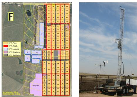
Figure 1. Map of the 30,000-head cattle feedlot and a photograph of the flux tower positioned at the northern edge of the operation. Fetch to the south, the prevailing wind direction, was 1600 m.
