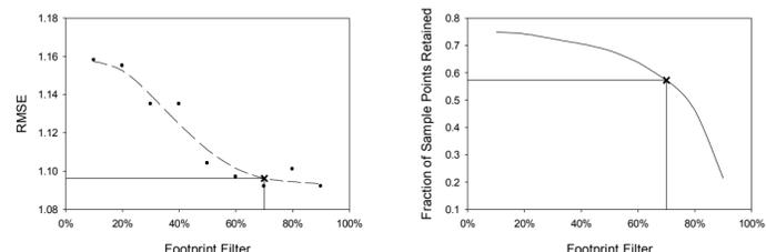
Figure 5. (a) Root mean square error between the expected and measured CO<sub>2</sub> fluxes as a function of the footprint filter criteria. (b) Fraction of the sample points retained at different filtering levels. An x-axis value of 70 represents a filter where flux data would be retained (i.e., considered valid) if the Hsieh model predicted 70% or more of the flux originated within the boundaries of the feedlot.
