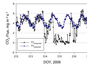
Figure 4. Example of measured CO<sub>2</sub> fluxes at the tower to the expected CO<sub>2</sub> flux from the cattle pens during a 5-day period. Deviations between the measured and expected flux indicate the tower was sampling outside the feedlot.
