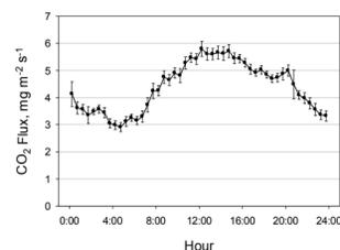
Figure 3. Composite graph of the diurnal CO<sub>2</sub> emissions from the feedlot. Data were filtered to only include periods when the winds were from the south and the source area was centered over the pens (Fig. 3).
