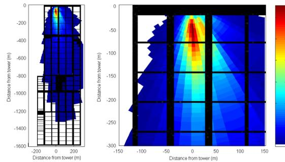
Figure 2. Contour plots of the source area footprint when wind direction was southerly.
