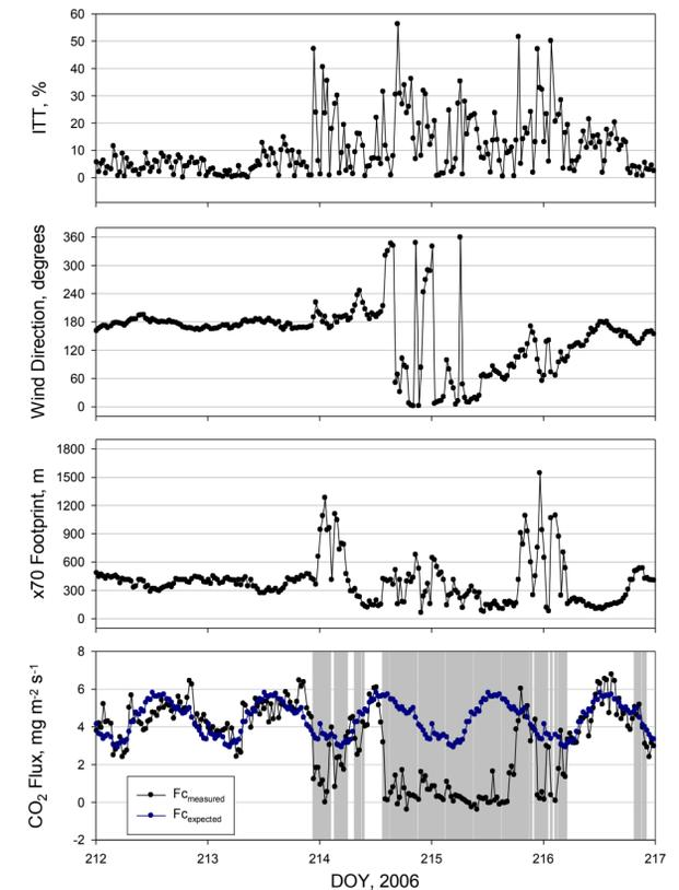
Figure 6. (a) integral turbulence test, (b) wind direction, (c) x70 footprint calculations, and (d) measured CO<sub>2</sub> flux versus expected CO<sub>2</sub> fluxes, with the gray areas representing periods where test(s) failed and sampling ceased.
