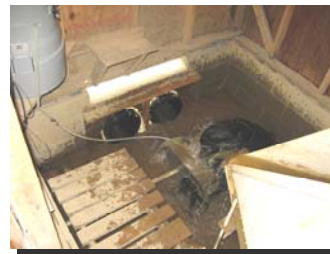
Flume, Sampler, and Culvert Diversions in Samplers and Filter Socks in Lower Waterway of Watershed 118
