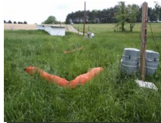
Flume, Sampler, and Culvert Diversions in Samplers and Filter Socks in Lower Waterway of Watershed 118
