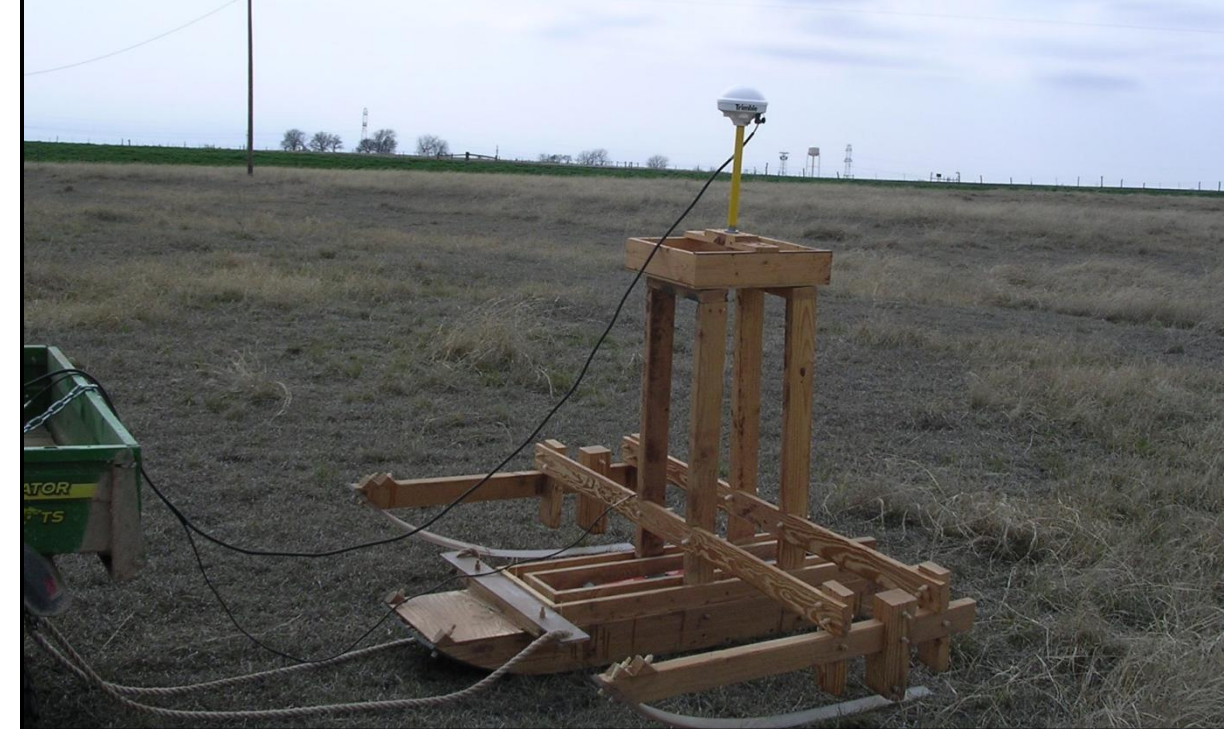
Fig. 1 Conducting a bulk soil electrical conductivity (ECa) survey prior to planting
