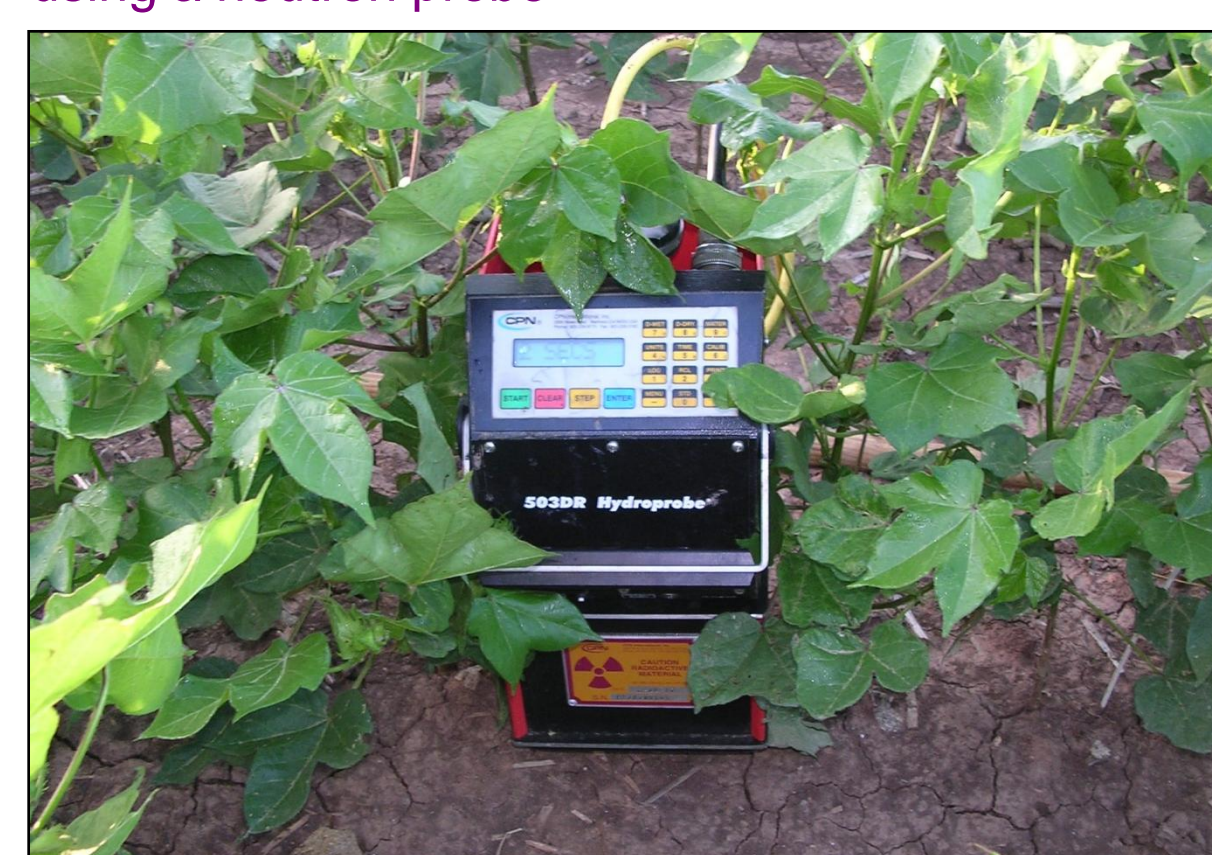
Fig. 4 Soil water content profile measurements using a neutron probe
