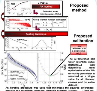
An iterative procedure was used that minimizes the squared differences between the measured reference retention function (RefWRC<sub>meas</sub>) and the reference soil water retention functions as obtained from the AP-model (RefWRC<sub>AP</sub>),
