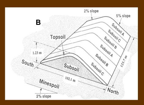
Figure 1. A. Structure of double wedge reclamation site near Zap, ND. B. Plan of replicated subsoil quality areas on wedge.
