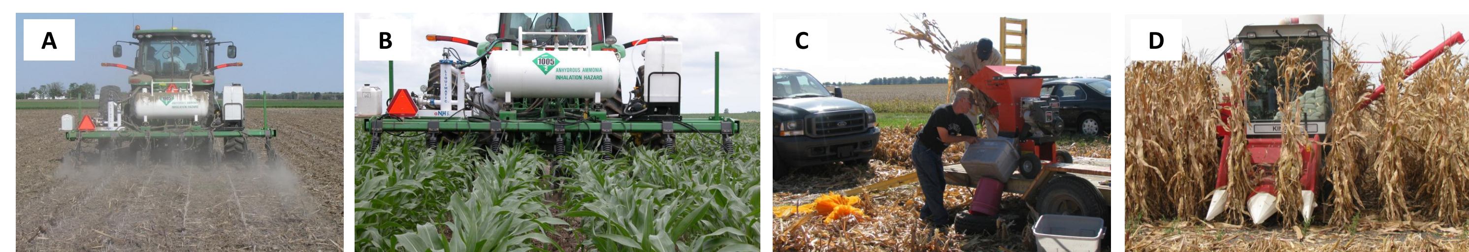
Figure 1. (A) Pre-plant NH 3 application 15-cm offset from future corn row; (B) side-dress NH 3 application in mid-row position; (C) biomass harvest at physiological maturity; (D) machine harvest in the center 2 rows
