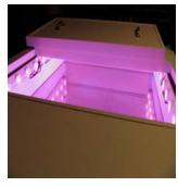
Thermogradient table with cover partially removed revealing the aluminum plate where the temperature gradient is maintained. LED grow lights provide light in the photosynthetic range without adding significant heat to the system.
