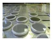
Gradient tables are well suited for Petri dish experiments where samples must be incubated over a range of temperatures simultaneously.
