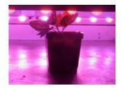
Small potted seedlings can be grown on the gradient table although the gradient dissipates above the aluminum plate surface.
