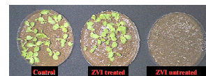
Fig. 5 Effects of ZVI treatment on the germination rate and growth of Lactuca sativa L. grown in the metolachlor contaminated soil.
