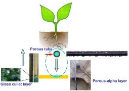
to prevent salt accumulation by the groundwater rising Upward flow by the capillary rise was stopped by capillary barrier using cullet as shown in left picture.
