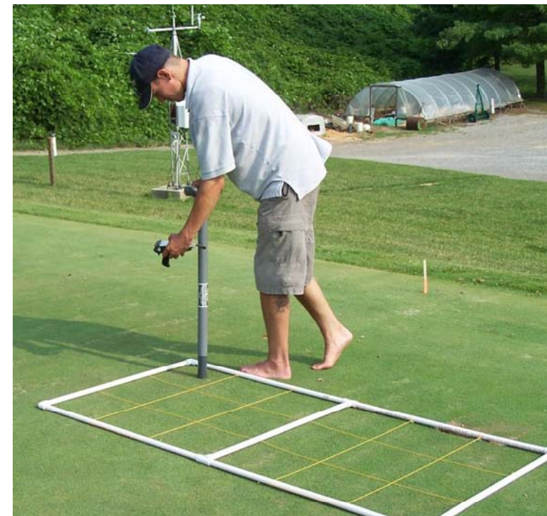
Figure 1. Use of the ML2 ThetaProbe and grid to take 18 volumetric soil moisture (0-4 cm) readings per plot
