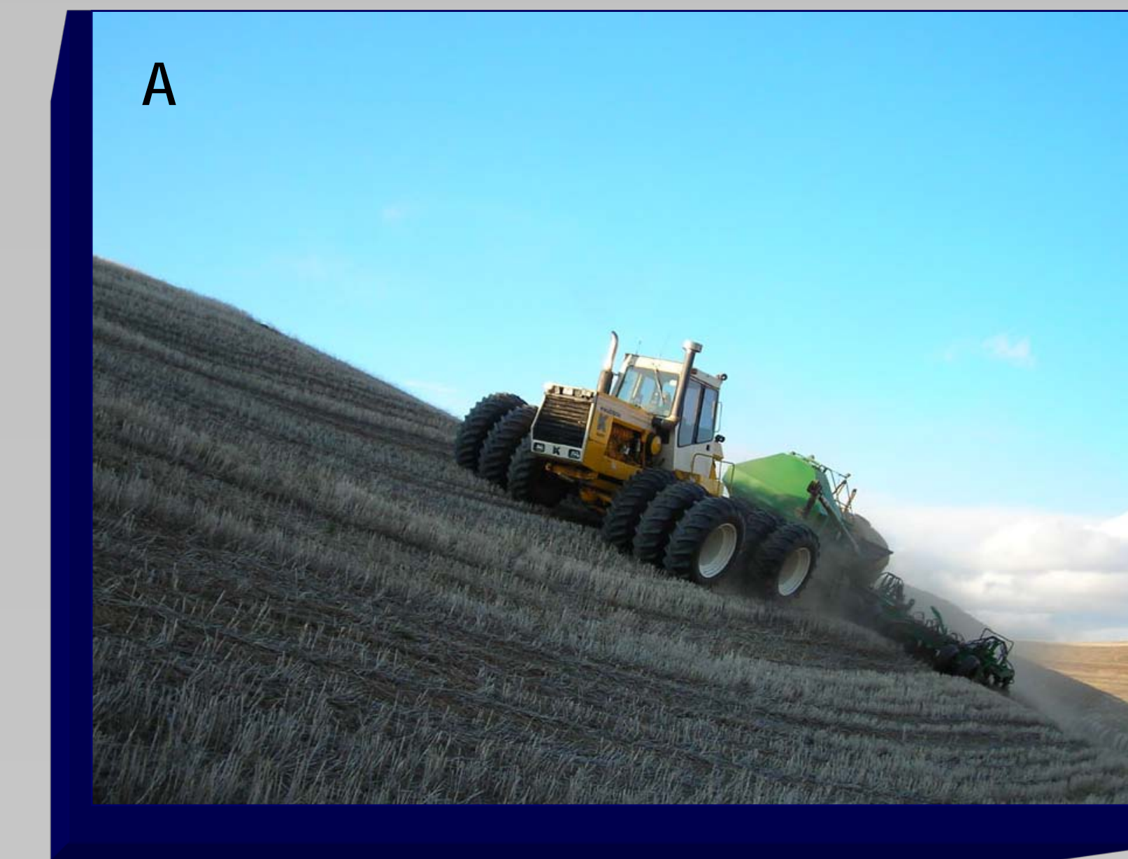
Fig. 3b. The 12-m-wide modified Great Plains model 3010 air drill has a notched coulter in front of each seed opener to cut through residue and 2-cm-wide shanks to band liquid aqua NH 3 -nitrogen plus thiosulfate-sulfur about 8 cm below the soil surface. Liquid "starter" fertilizer from a separate tank delivers phosphorus close to the seed that is planted with double-disc openers on 20 cm row spacing. This field has been in continuous no-till for 30 years. Photos by John Aeschliman, Colfax, WA.
