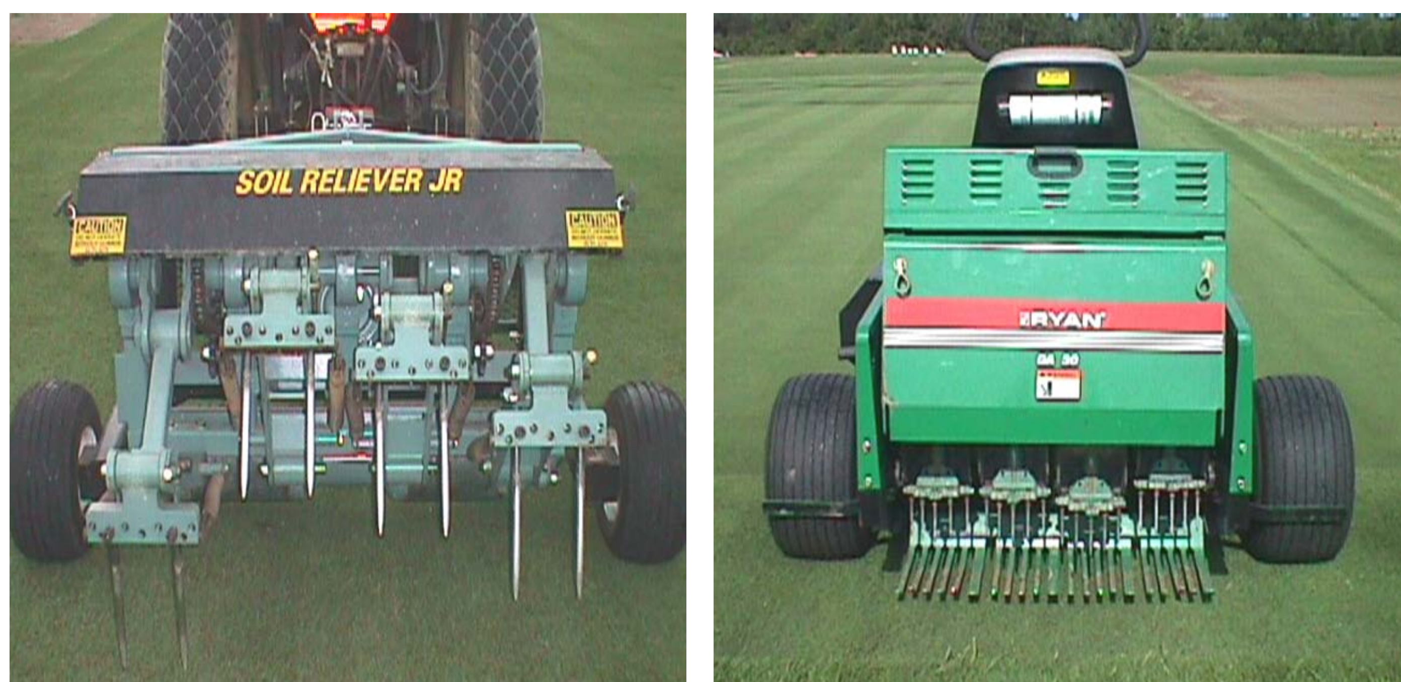
Figure 1. Aerification equipment used to apply the treatments. Left, Soil Reliever ® used for the deep-depth tine treatments (DST shown), and, right, Ryan ® aerifier used for the standard tine treatments (SST shown).
