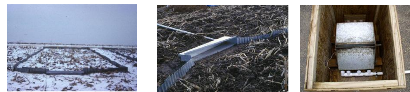
Runoff sampling: plot (left); runoff collector (center); tipping pan and sub-sampler (right)
