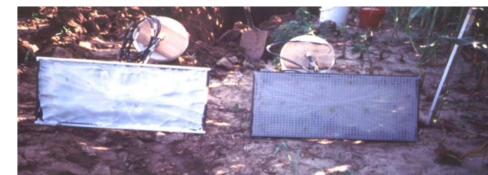
Percolation water sampling: pan lysimeter (left); wick lysimeter (right)
