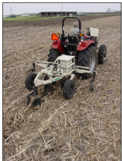
Fig.1 Veris NIR Spectrophotometer (Shank)
