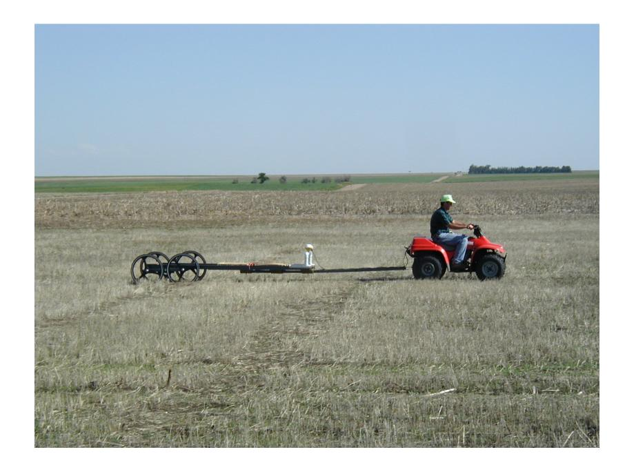
Figure 1. Equipment used to collect ECa data.
