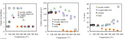
Fig.5 Water repellency, total carbon content and C/N ratio of soils after muffle furnace burning.
