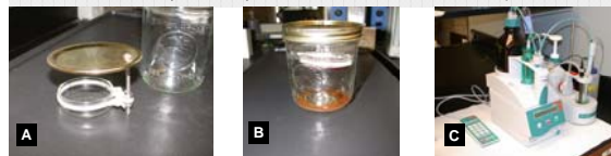
Figure 1. (A) Diffusion unit used to measure soil amino nitrogen content using the methods of Kahn et al. (2001). One g of soil is added to the mason jar with 10 mL of 2 N sodium hydroxide. (B) A petri dish suspended from the jar lid contains 5 mL of boric acid (4% w/v). The unit is placed on a hot plate at 50°C for 5 hours. (C) After heating, the petri dish is removed, 5 mL of distilled water is added, then the solution is titrated with 0.02 N H 2 SO 4 . Amino N content is calculated as S \times T = \text{amino N PPM} , where S is the volume of H 2 SO 4 and T is the titer (280 μg mL -1 for 0.02 N H 2 SO 4 ).
