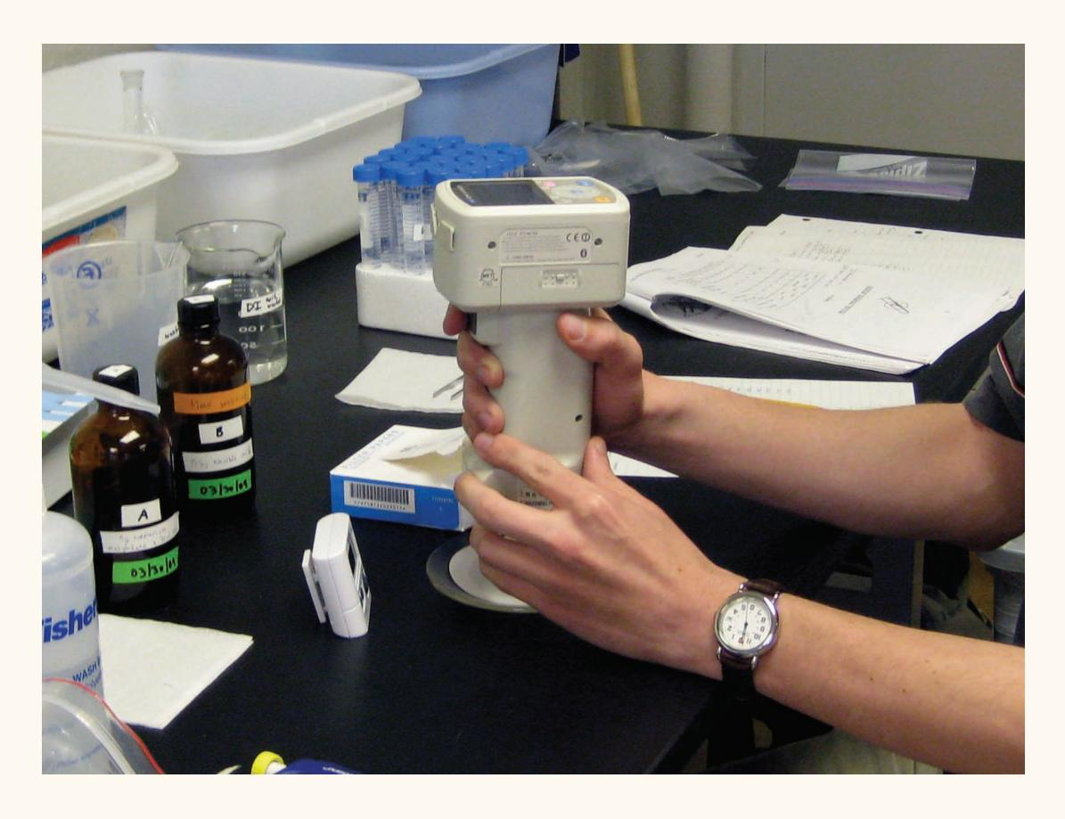
Konica-Minolta **VIS-reflectance** spectrophotometer
