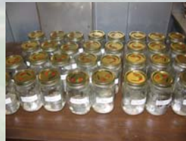
Fig. 3. Each core was incubated at 25°C in a 1000 mL Mason jar together with a \text{CO}_2 -trap (10 ml 2M NaOH).
