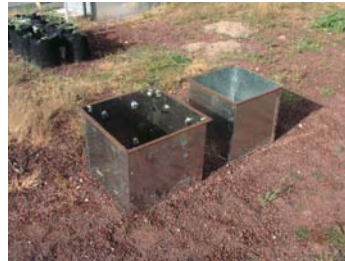
Figure 1. The metal boxes. The inside box contains the soil and is balanced by metal springs: up & down, as the soil water changes.
