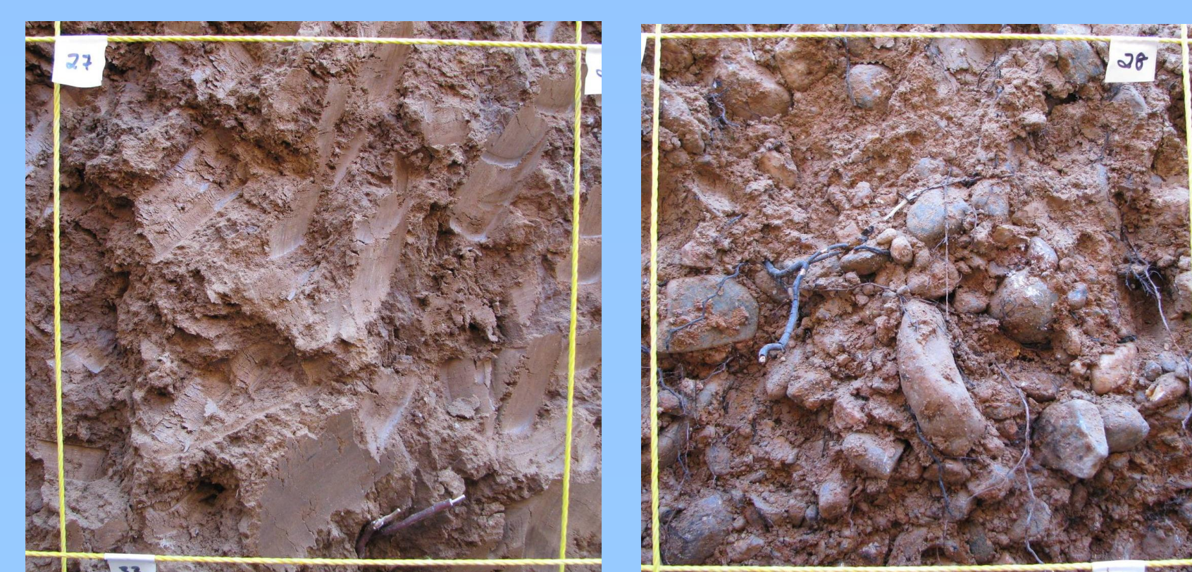
Figure 2. Contrasting soils in the Rancho Seco vineyard. Left: Soil 2.1, loamy topsoil over very clayey, compact subsoil with few gravels. Right: Soil 2.2, gravelly sandy loam with 75-83% coarse fragments.
