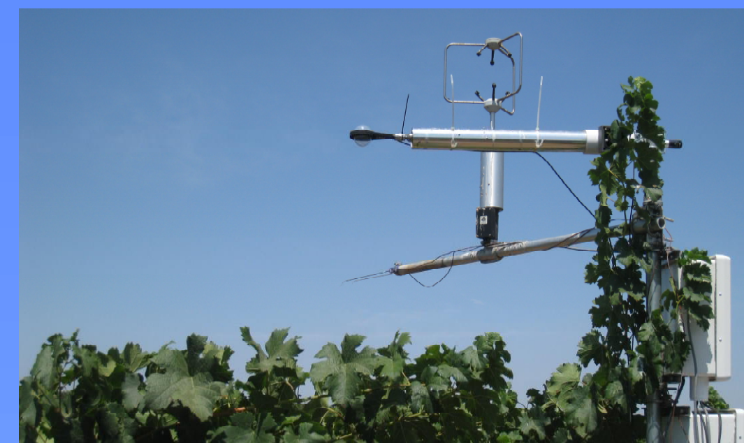
Figure 1. Surface renewal station. Thermocouples are shown extending to the left from the station. The 3-d sonic anemometer is on the same arm as the thermocouples. The net radiometer (Rn sensor) is in the foreground. In addition, 3 soil heat flux plates are buried at 5 cm depth, one in the row and the others at 1/3 and 2/3 distance between rows. Soil temperature probes were inserted in the 5 cm soil layer at 12 locations to obtain the mean change in soil temperature over half hour periods. In conjunction with the heat flux plates, the change in soil temperature is used to estimate a mean value for soil heat flux on the ground surface.
