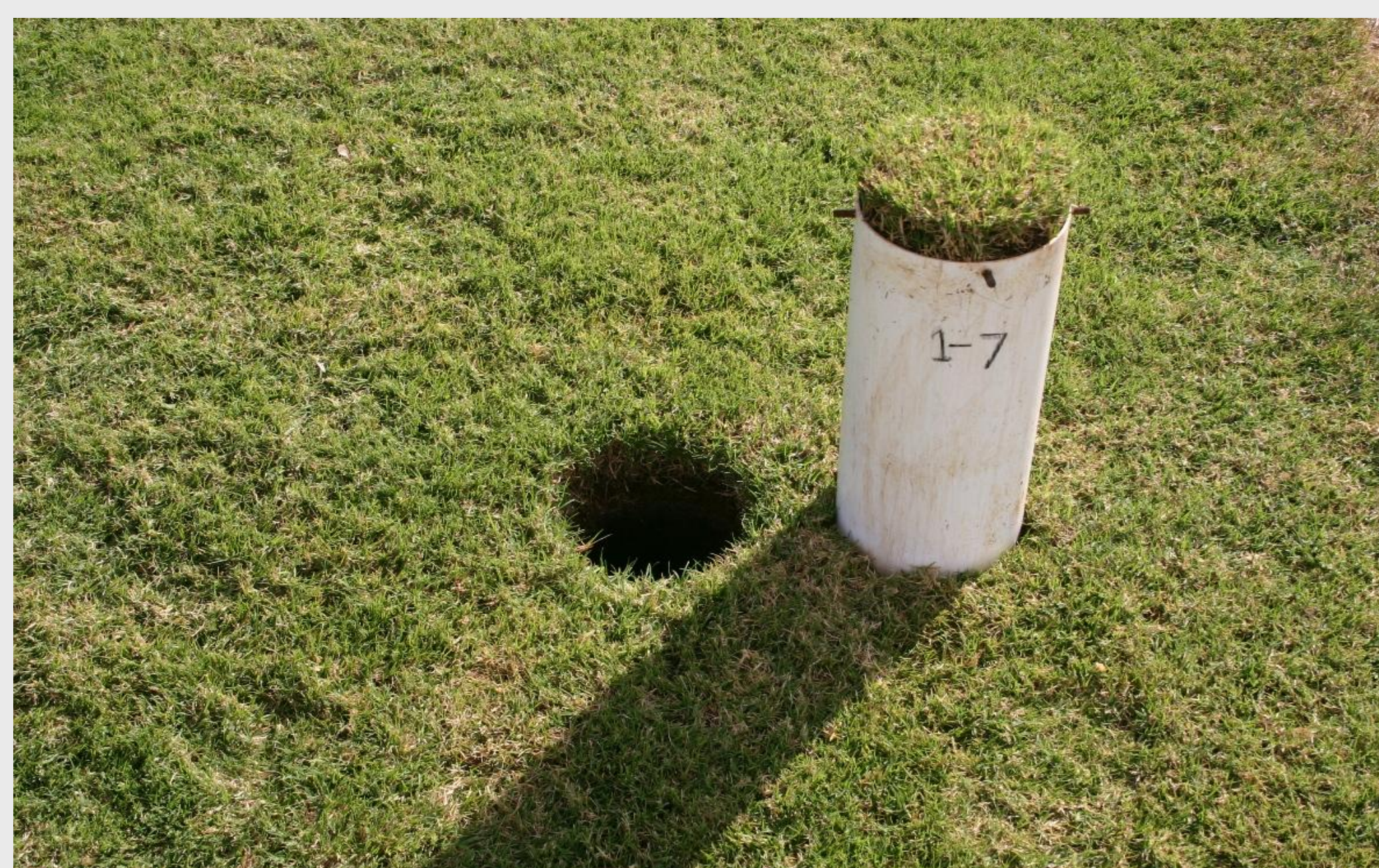
Figure 2. Mini-lysimeter shown removed from its respective turfgrass plot.
