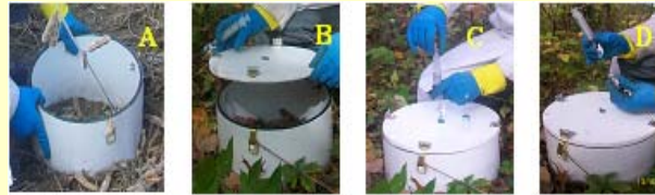
Figure 2. Installing the chambers (A), closing the lids to begin gas flux measurement (B), taking a gas sample (C), and storing air sample in a vial until analysis by gas chromatography (D).
