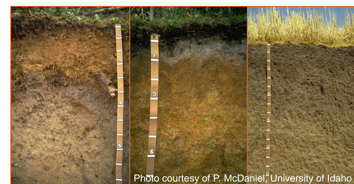
Figure 2. From left to right: forest Andisol, forest Spodosol, agricultural Mollisol Photo courtesy of P. McDanel, University of Idaho
