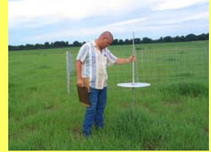
Forage Yield (Fresh) Measurement using Drop Height Technique
