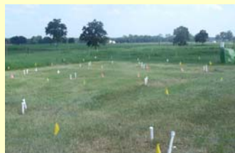
Figure 2. Experimental field showing Tifton-85 and suction lysimeters.
